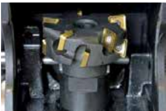
Mono block milling head, with 10 indexable inserts fixed with screws.
