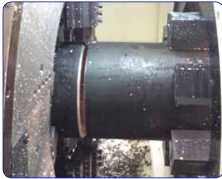
Double hydraulic clamping system front and rear of cut
